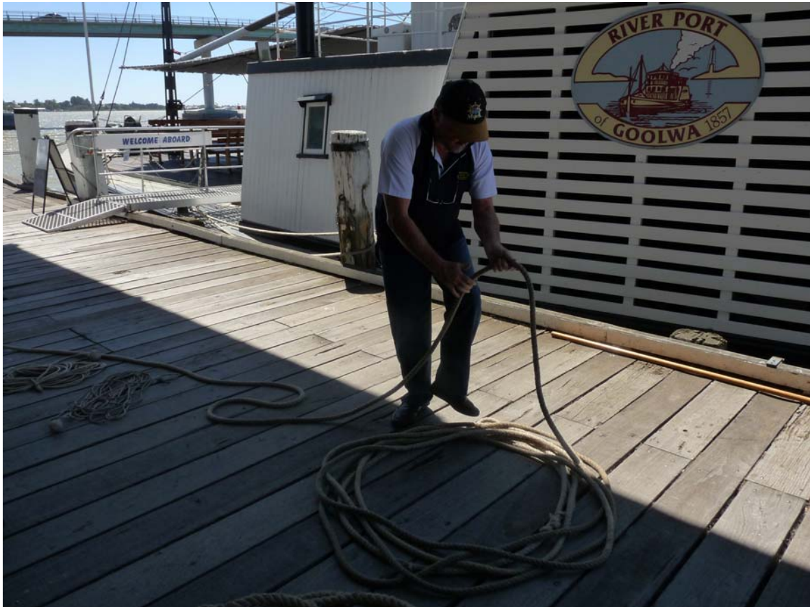
Skipper E.J. demonstrates rope handling techniques, in this case correctly coiling or flaking a rope, preparatory to either stowing, or throwing in a mooring manoeuvre.
